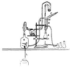
wet combustion with chromic and sulphuric acids. C is a tube, filled with solid potash, guarding the apparatus from the carbonic acid of the air. The small drop funnel B carries acid to the decomposing flask The small conden-Α. ser D returns most of the water vapor, and the hydrochloric acid to the decomposing flask. The
